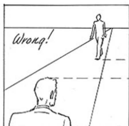
Wrong! These men could not be standing on the same Ground Plane.
